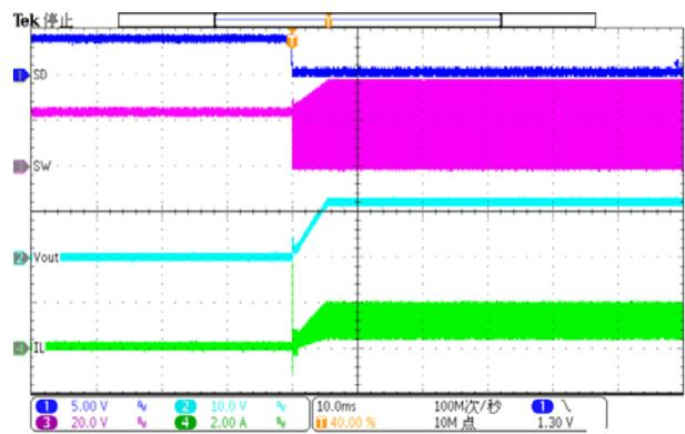
Figure 31. Shutdown remove
