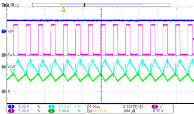
Figure 24. Steady-state (Iload=2A)
