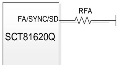
Figure15. Frequency Adjust
