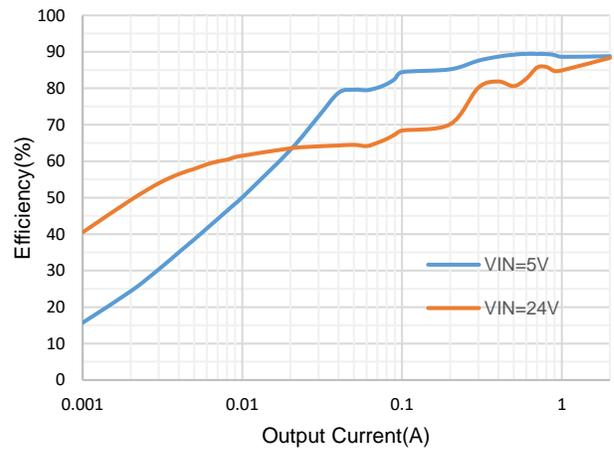
Figure 6. Efficiency vs Load Current, Sepic, VOUT=12V
