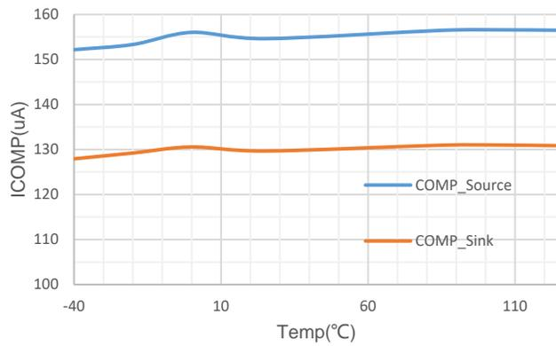
Figure 9. COMP Current vs Temperature
