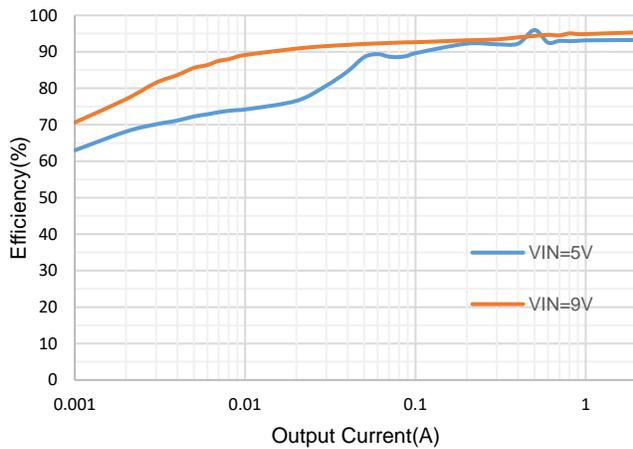
Figure 5. Efficiency vs Load Current, Boost, VOUT=12V
