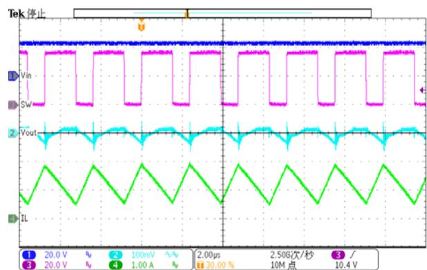
Figure 33. steady-state (Iload=2A)
